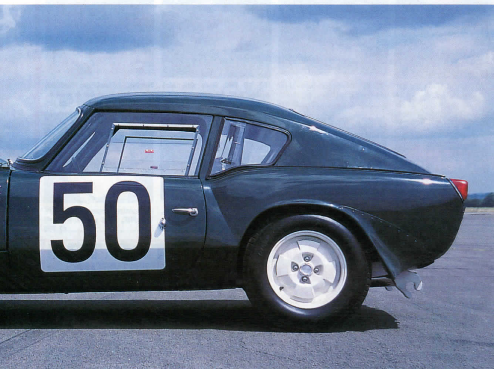
Left: Hard to believe, but Spitfire race replica was built because of a £10 autojumble purchase. Le Mans 5.5J x 13 inch magnesium wheels have since been copied for Jigsaw, tyres are Dunlop 5.50L - 13 radials
