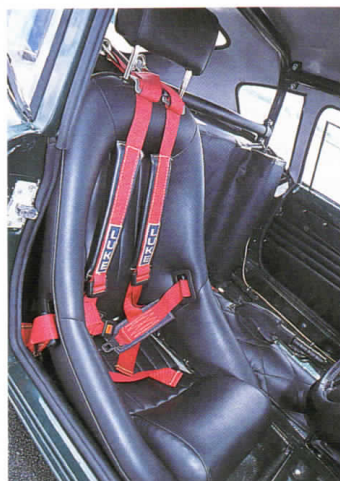
Above: Racing car interior is pretty sparse. Modern safety harness and specially-built seat are required to meet regulations. Note adjustable knee pad mounted on transmission tunnel and matching pad on door for driver comfort on long-distance event. Hole in dashboard is fresh-air vent
