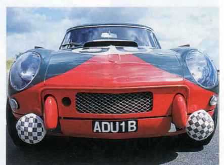
Left: Hard to believe, but Spitfire race replica was built because of a £10 autojumble purchase. Le Mans 5.5J x 13 inch magnesium wheels have since been copied for Jigsaw, tyres are Dunlop 5.50L - 13 radials
